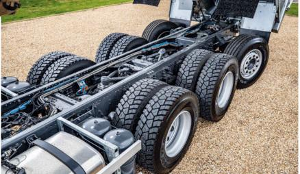
some competitors', is well-protected with steering arms tucked out of harm's way. This, along with the position of the rear air bags, makes it possible to tip into an asphalt paving machine without fouling, an important consideration for tippers.
